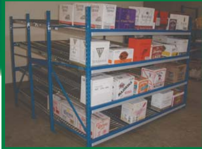
Full Case Pick, Double-Deep RollerRack Low Profile Span-Track throughout
