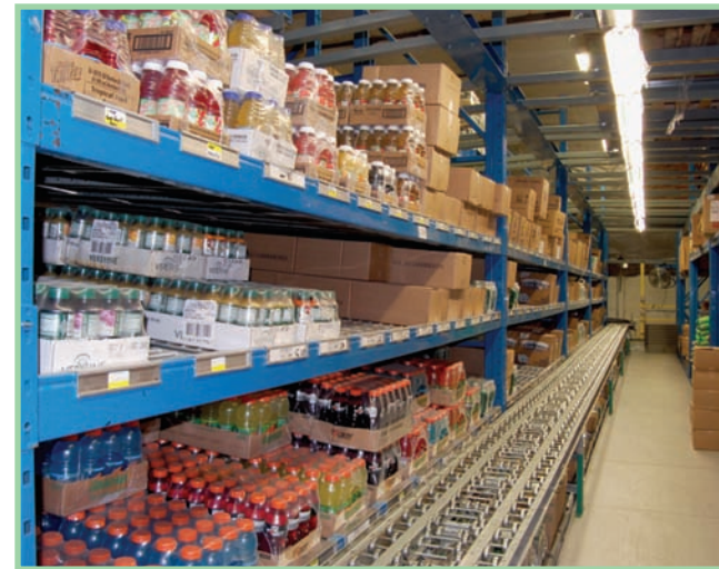
Low Profile Span-Track added to floor level of three story pick module, maximizing use of vertical space and assuring reliable carton flow.
