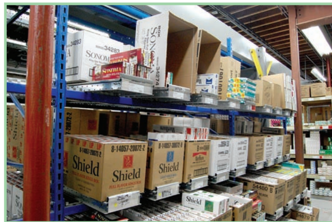
High Profile Span-Track extended beyond the beam optimizes use of linear space and delivers items right to the pick point.
