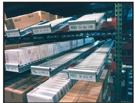
Middle: Unex Conveyors Move Product to Distribution. Bottom: Span-Track (High-Profile Model) Brings Cartons to Pickers.
