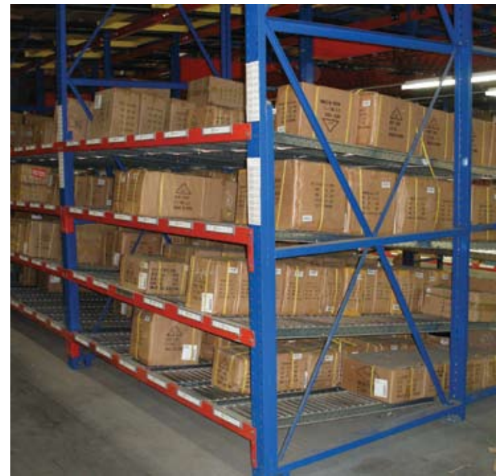
Span-Track full width rollers assist restocking from back of rack while feeding work to pickers in front. Picking is not interrupted and FIFO is maintained.
