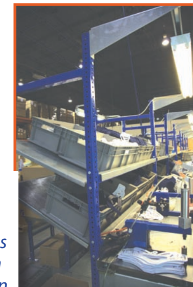
Flow Cell with Tilted Pick Shelf angles totes toward the worker making items easier to see and access.
