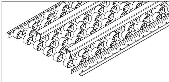
When installing guide rail on higher levels, ensure the end of the guide rail is visible at the edge of the charge end. This will provide the loader a visual cue of where to place the box.
