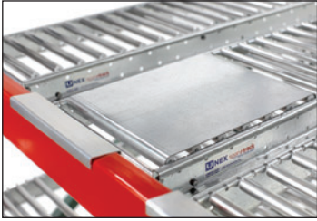
Impact/Slow Down Plate Steel impact plates snap over rollers or wheels at load end for impact or at pick end for friction slow down
