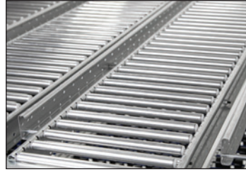
Guard Rail - Lane Guard rails that bolt onto the side of the track. 4 spacer widths available with in- or out-flange configuration.
